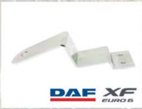
TB-40 STAINLESS STEEL TRUCK BRACKET 3mm, ELECTRO-POLISHED FOR DAF. It is installed with rivets above the driver's side door
